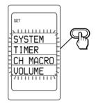
"TIMER" appears on the LCD display, and the timer program numbers are displayed on the labels. To change the labels (PROG 1- 12), press the SCROLL button repeatedly.
